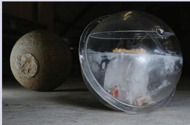
An example of a passive smart rock containing a magnet suspended in liquid is in the foreground. Active smart rocks have embedded electronics. In the background is a concrete-encased smart rock that is about the size of a basketball and weighs about 50 lbs.
