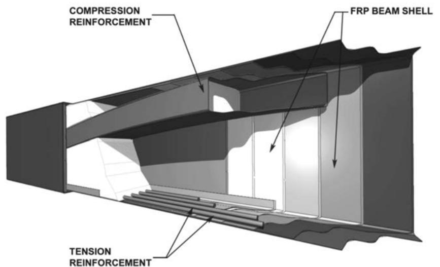
**Tucked inside durable, fiberglass composite shells, the lightweight beams are supported by a concrete arch and anchored by seven wire tendons, which serve as the system's tension tie.**
