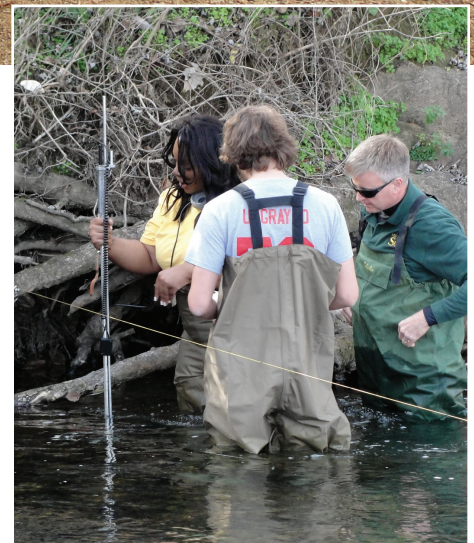
Adjunct professor Robert Holmes and CE234 students at the Little Piney River near Newburg, Mo., conduct streamflow measurements.
