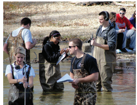
Adjunct professor Robert Holmes and CE234 students at the Little Piney River near Newburg, Mo., conduct streamflow measurements.
